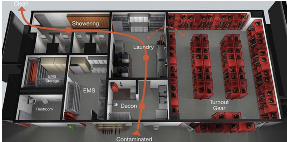
3 Mitchell Associates Architects designed this large decon area, laundry, showering area, and turnout gear storage area for the Southbridge (MA) Fire Department. (Photos 3-5 courtesy of Mitchell Associates Architects.)
