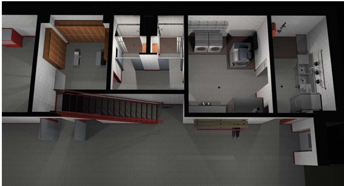
4 Decon areas can be relatively compact, as show in this layout designed by Mitchell Associates Architects for the Selkirk (NY) Fire Department.
